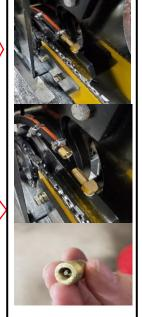
1) Remove brass manifold located by bar/chain
