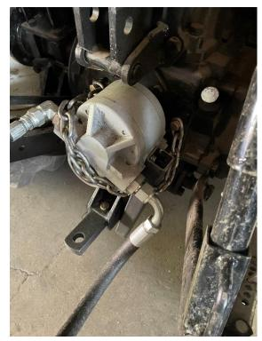
Ensure the support brace is orientated correctly to prevent PTO pump from spinning.
